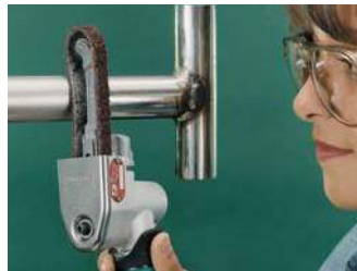
Clean and finish using non-woven nylon belts.
