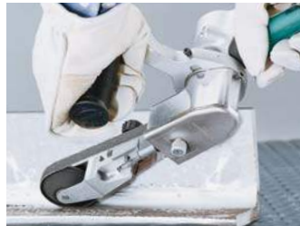
Utilized for blending scratch patterns and grinding right angle welds.
