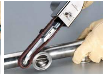
Clean and finish using non-woven nylon belts.
