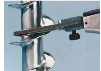
Clean and finish using non-woven nylon belts.
