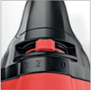
Continuous pendulum stroke adjustment (only for RSP 13-32) From 0-3 mm, to speed up progress when working on non-metal materials
