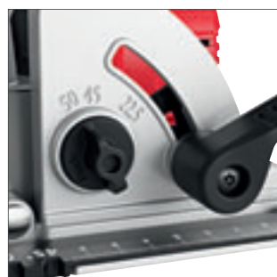
Doubly clamped swivel segment from 0° - 50° With pre-selection function for angles of 22.5° / 45° / 50° to provide safe, precise guidance of the saw when making angular cuts. Prevents the saw blade from jamming in the material.
