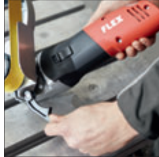
Clamping lever Position of tool and handle can be varied
