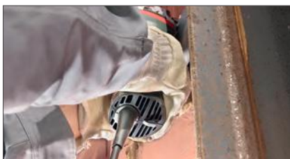
Rear vents: Optimize air flow for cooler operation
