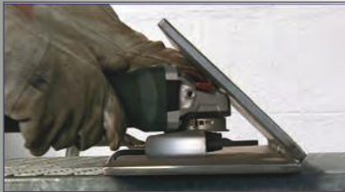
Typical problem...Grinder doesn't reach
