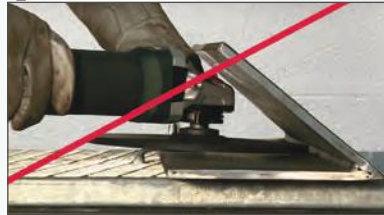
Typical solution violates safety standards
