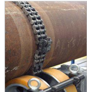
Adjustable chain (ø 8" – 40") ensures positive axial rotation
