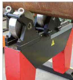
Optional heavy-duty pipe support with 11-ton capacity
