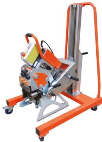
3D Trolley features vertical height adjustment and floating compensation for uneven floors
