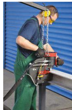
Overhead Support for Punch SM-ZUR-0517-15-00-00-0 Integrated overhead boom support allows for easy manipulation of punch and power pack as single unit.
