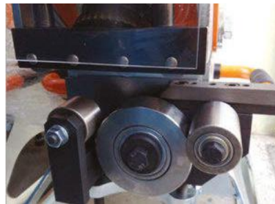
Extra wide guide rollers for easy alignment to the plate
