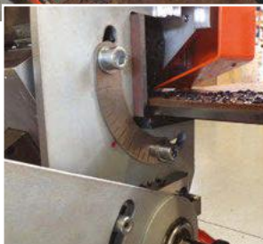
Rapid 180° inversion for bottom side bevel
