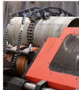
Clamping device for short pipes of 15-3/4" – 32-11/16" length
