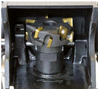
Mono block milling head, with 10 indexable inserts.
